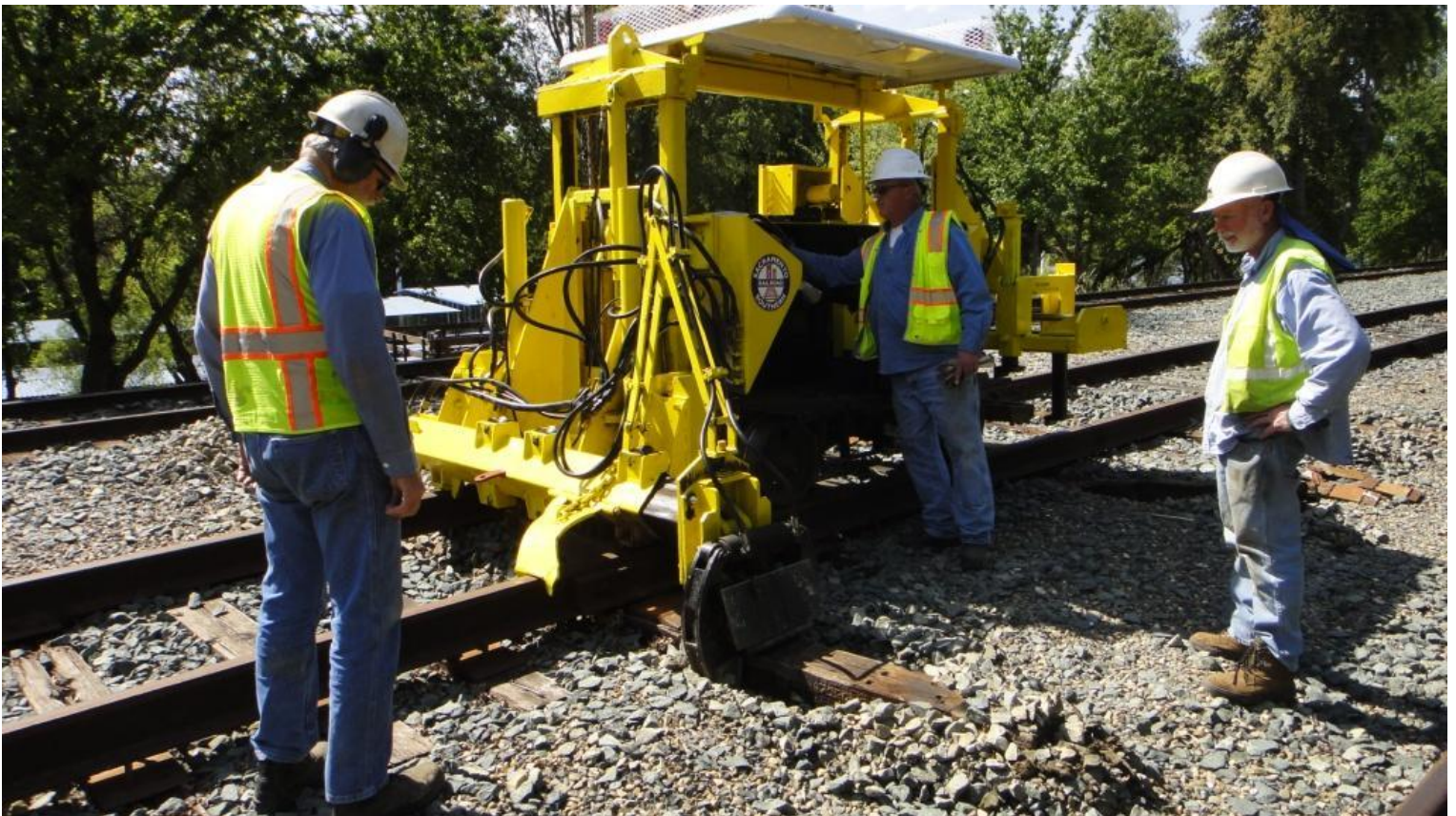
Having lowered the work-head and, after making adjustments to the hydraulics, Scott tests the 125's rail-clamping systems
