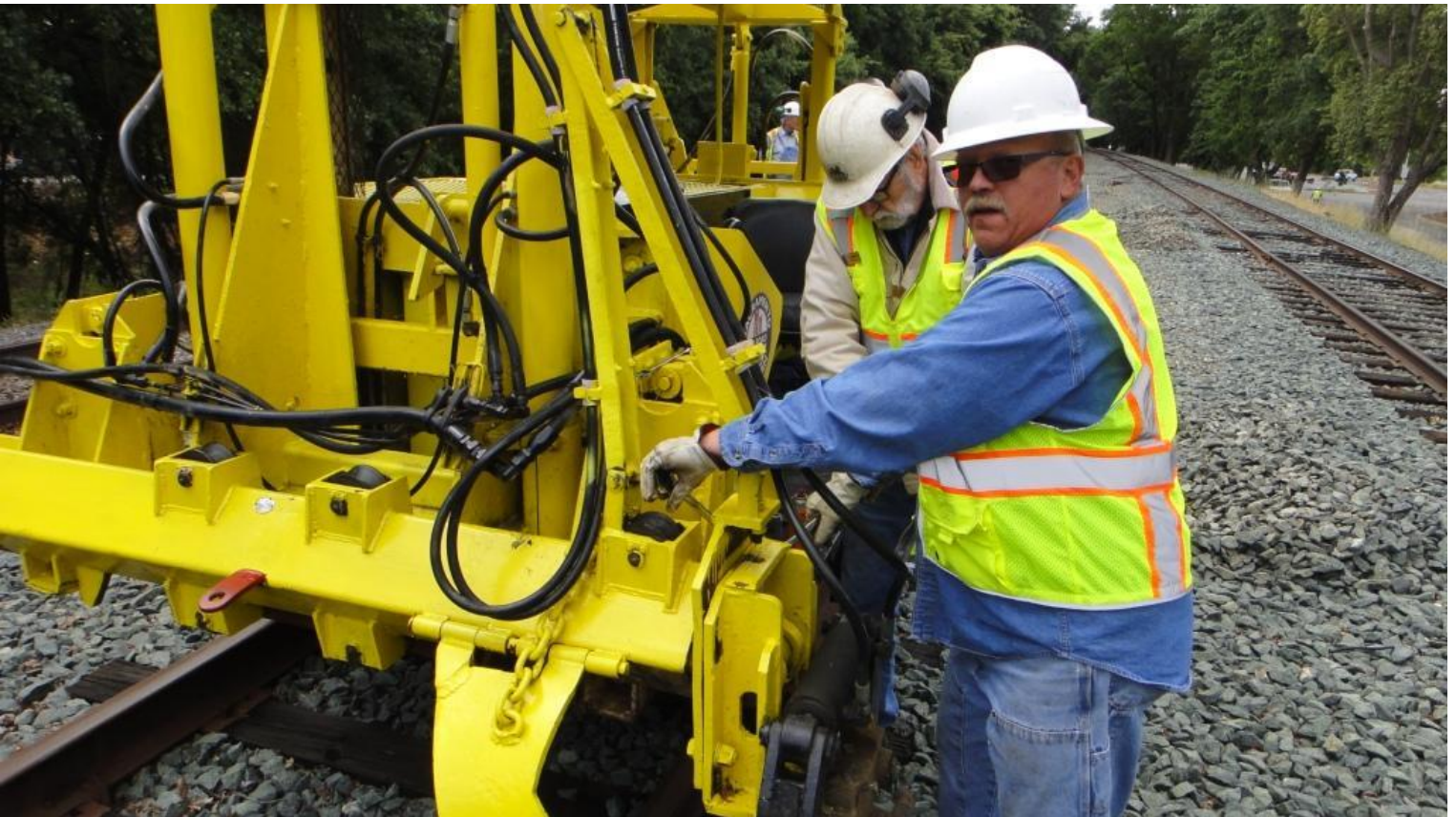
Scott makes adjustments to the work-head height
